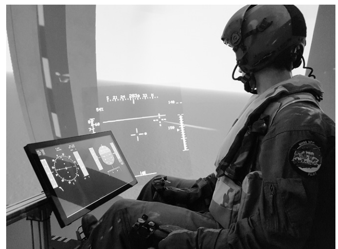
Fig. 1. Simulator setup of the generic helicopter cockpit inside a dome projection with head-slaved helmet-mounted display (HMD) projection.
