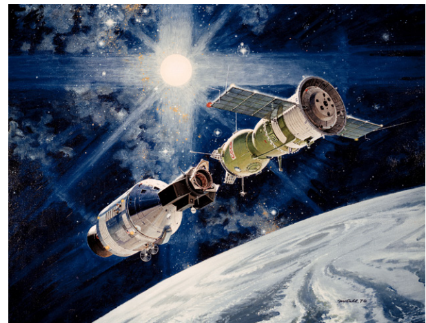
Fig. 1. An artist's rendition of the Apollo spacecraft about to dock with the Soyuz using the multipurpose docking module, which allowed transfer between the spacecraft despite the disparate atmospheres (NASA/Robert McCall).
