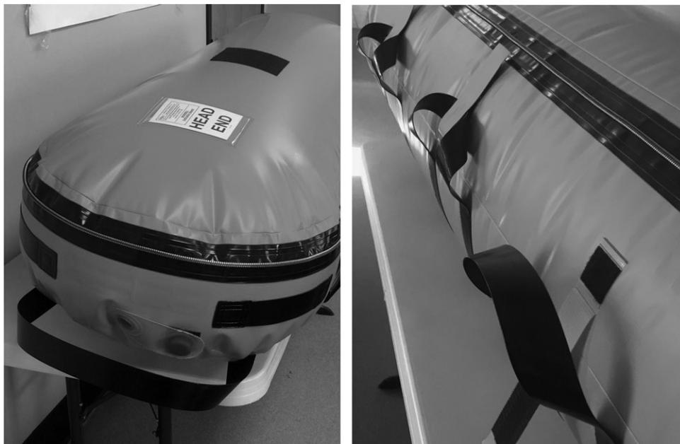
**Fig. 1.** Modified HRCU, including reinforced zipper with reverse orientation and opening at the head (left) and the addition of securing straps to handling loops along the length of the unit (right).
