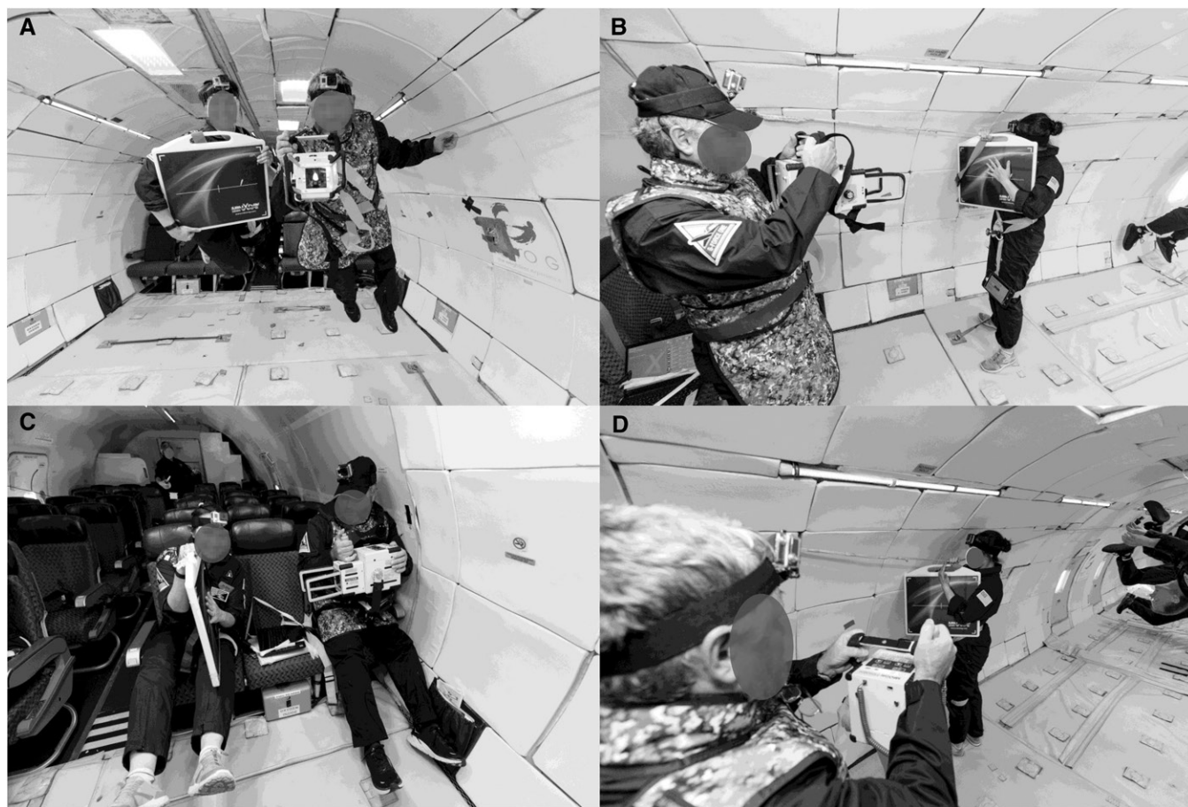
Fig. 1. A) Two of the authors pose in microgravity aboard a parabolic flight with the ultra-portable x-ray generator and image receptor. B, C, D) Example image acquisitions of the two technicians in various positions. Photo credit: Steve Boxall, Zero Gravity Corp., 2022.
