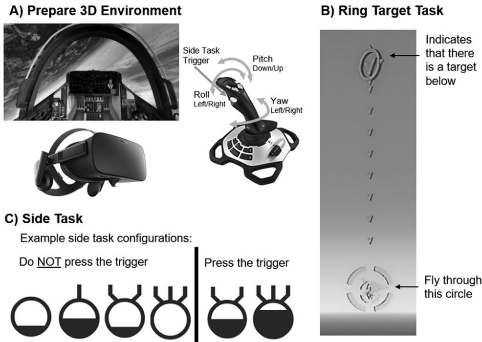
**Fig. 1.** (A) Prepare3D flight simulation program in the VR environment displayed in the Oculus headset and controlled by the Logitech Freedom 2.4 GHz joystick. Joystick movements in pitch, yaw, and roll axes performed the Ring Target Task and the pointer finger trigger button on the joystick performed the secondary task. (B) Primary Ring Target task during the flight simulation in the VR environment. (C) Secondary task in the field of view during the flight simulation.
