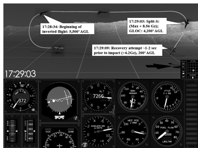
Fig. 2. Mishap pilot during the high bomb burst rejoin maneuver on the day of the mishap. MA parameters across the bottom of the figure correspond to the maximum +G_z during the Split-S, at 17:29:03 UTC (1 s prior to G-LOC). Top row, left to right: airspeed (372 KCAS); altitude indicator: approx. 90^\circ nose low and 5\text{--}10^\circ left bank; altimeter: 7266 ft MSL (4266 ft AGL); engine RPM: 82%; turbine inlet temperature (FITT): 690^\circ\text{C} . Bottom row, left to right: angle of attack (AOA): 16.5 ; vertical velocity indicator (VI): descending at 39,700 \text{ FPM} ( \text{ft} \cdot \text{min}^{-1} ); heading indicator: 234^\circ (west-southwest); acceleration G units: +8.6 G_z ; engine nozzle position (NOZ POS): 21% open; fuel flow: < 1000 \text{ lb} \cdot \text{h}^{-1} (normal for idle power). Far right, top: throttle setting: idle power; stick position: aft stick; rudder position: neutral. Far right column: caution/warning panel: no cautions or warnings illuminated.
