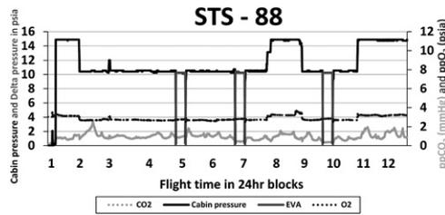
**Fig. 2.** Example of a shuttle mission’s timeline depicting cabin pressure (solid black line), three EVA times (solid dark gray lines), ppO<sub>2</sub> (dotted black line), and ppCO<sub>2</sub> (dotted light gray line). This figure shows an interrupted 10.2-psia depressurization after about 8 d.
