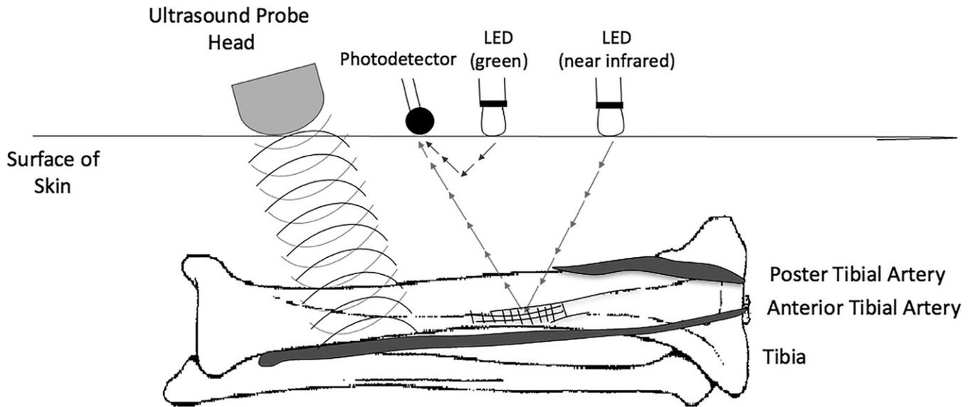
**Fig. 1.** Visual schematic of anterior tibial artery macrovascular blood flow detection using ultrasound technology and tibial bone microvascular blood flow detection using the photoplethysmography (PPG) device.
