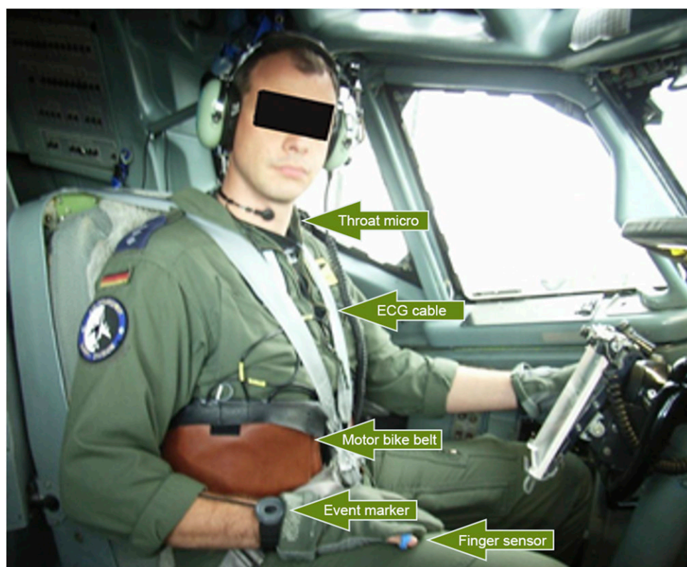
Fig. 1. Measurement equipment during simulator and real flights.
