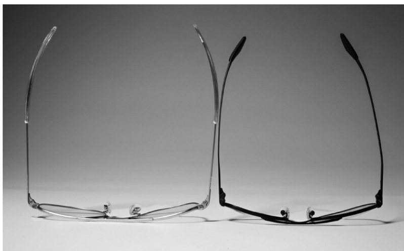
Fig. 4. Top view showing face form angles of current modified HGU-4/P Apache aviator frame (left) and USAARL prototype Apache aviator frame (right).
