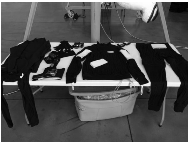
Fig. 1. Undergarments, including thermal underwear, physiological monitor, and integrated cooling system. Padding (white blocks) were used to prevent pressure points.
