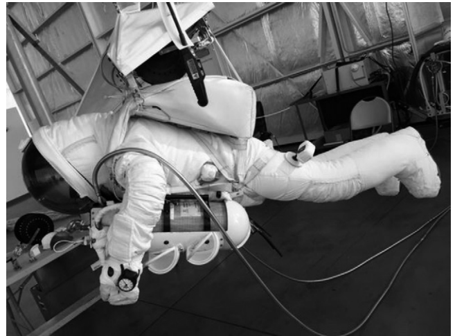
Fig. 2. Pressure suit assembly with anterior life support and posterior parachute. Two silver hoses are ground oxygen lines removed prior to flight.
