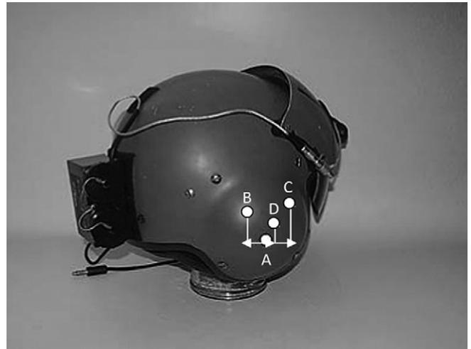
**Fig. 1.** The centers of gravity in each testing configuration: A) HEAD; B) HELMET; C) NVG; D) NVGcw.
