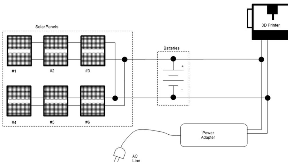
**Fig. 1.** Six 9V solar panels deliver 27V into an improvised voltage regulator that outputs a constant 24V to charge two lead-acid 12V batteries (5Ah, 18Ah) in series which provide the energy storage necessary to deliver the required current to operate the FDM 3D printer for less than 1 h/d.
