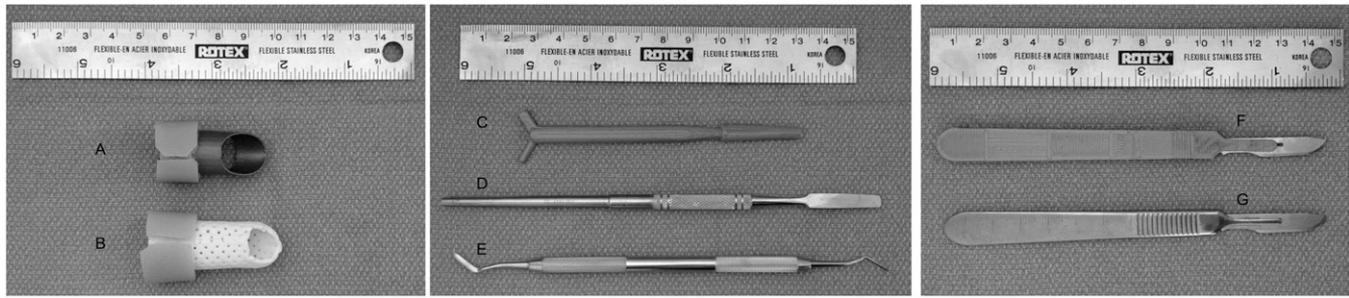
**Fig. 2.** Left panel: A) 3D printed ABS thermoplastic custom mallet finger splint, and B) handmade thermoplastic custom mallet finger splint. Middle panel: C) 3D printed ABS thermoplastic dental filling replacement tool, D) conventional stainless steel dental spatula, and E) conventional stainless steel dental plastic filling instrument. Right panel: F) 3D printed ABS thermoplastic scalpel handle with #10 blade, and G) conventional stainless steel scalpel handle with #10 blade.
