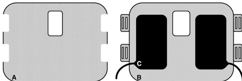
**Fig. 1.** Illustration of the components used in the sandwich design seat pan which allowed for pressure application during testing. A) Sitting surface (constructed of wood); B) nonmovable base with locations for strapping (constructed of medium density fiberboard); C) air bladders used to provide pressure connected to a MRI-compatible pneumatic modular robot controller (not shown).
