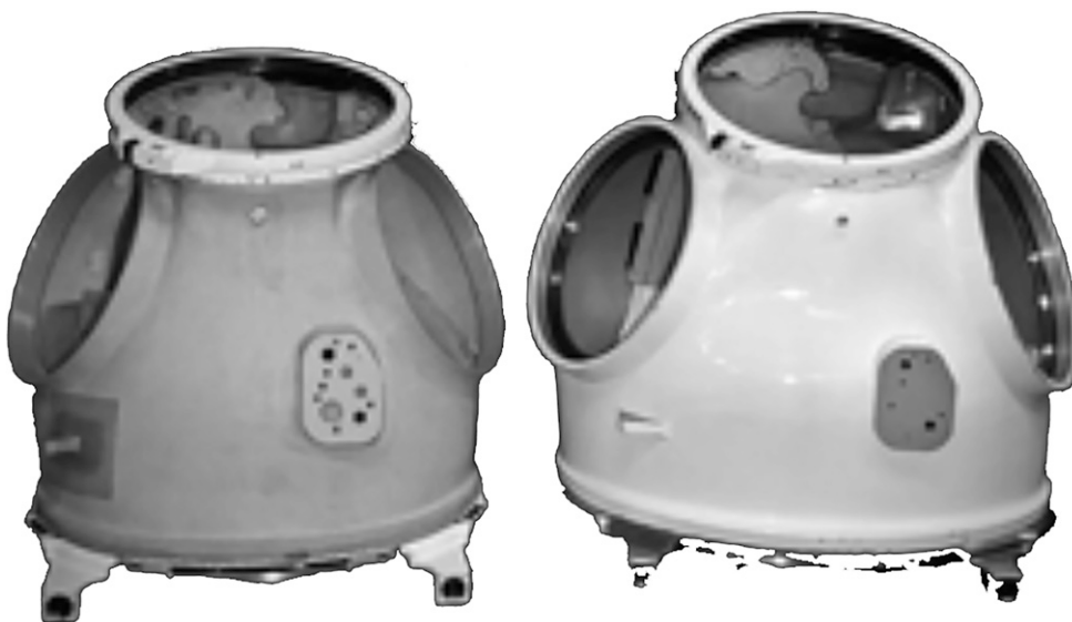
Fig. 1. Pivoted and planar hard upper torso (HUT) styles. There are two HUT styles with their primary difference being the shoulder scye bearing to which the arm components attach. The pivoted HUT, shown on the left, has a pivoting bellows to allow for greater shoulder mobility than the planar HUT, shown on the right. Photo credit NASA.
