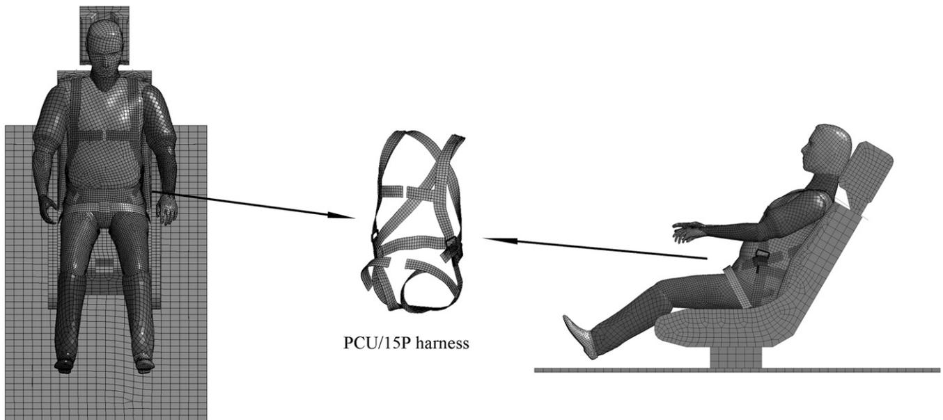
Fig. 1. Model of the mannequin and PCU-15/P harness used in the experiment.
