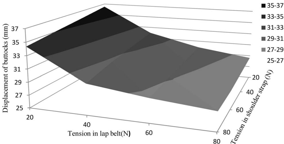
**Fig. 4.** Displacement of upper torso and lower torso of the mannequin with different tension values in the lap belt and shoulder strap under impact in the  $-G_z$  direction.
