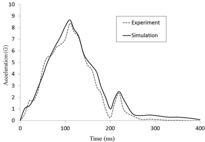
**Fig. 3.** Comparison of chest acceleration during  $-G_x$  impact in the simulation and Buhrman et al.'s experiments.<sup>4</sup>
